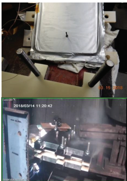
Figure 11: Nail penetration test pictures of 46Ah LMO/LTO cell. Cell was charged to 2.7V @ 46A tapered to 2.3A and placed into Nail Penetration fixture.
