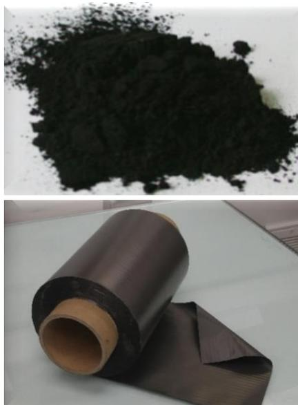
**Figure 1.** Dry powder mixture comprised of active materials, conductive carbon and polymer binder (top) and a roll of free-standing dry coated electrode film fabricated from a pilot scale roll-to-roll equipment (bottom).
