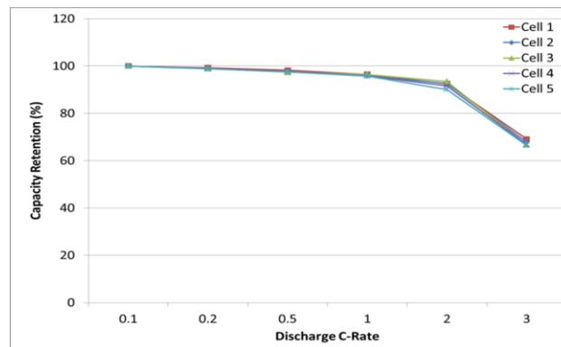
**Figure 5.** Rate performance of dry coated NMC111 (94 wt.% loading)/graphite (96 wt.% loading) electrode in prototype pouch cell: NMC111 electrode loading is 27 mg/cm<sup>2</sup> (4mAh/cm<sup>2</sup>). The cell was charged to 4.2V at constant current followed by constant voltage at 4.2V and discharged to 2.8V.
