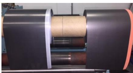
**Figure 2.** Dry battery electrode NMC roll (left) and graphite roll (right) double sided laminated onto current collector which is ready for cell assembly.
