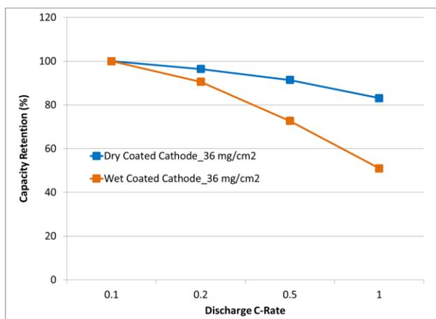
**Figure 4.** Discharge rate performance of dry coated NMC111/graphite full-cell in comparison to wet coated NMC111/graphite full-cell. Electrode loading is 5mAh/cm<sup>2</sup>. Cut-off voltage was 4.2V and 2.8V for charge and discharge, respectively.
