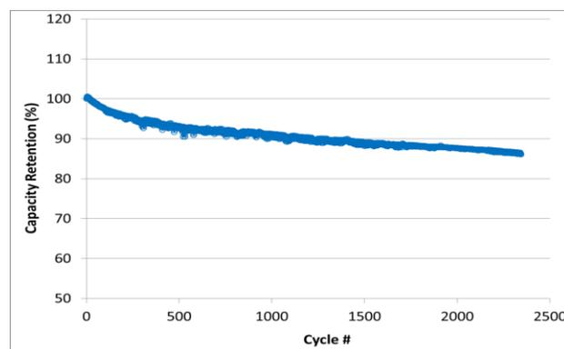
**Figure 6.** Cycle performance of dry coated NMC/graphite electrode in a prototype pouch cell at constant current 0.5C charge/1C discharge: Electrode loading- 4mAh/cm<sup>2</sup>. Cut-off voltage was 4.2V and 2.7V for charge and discharge, respectively.
