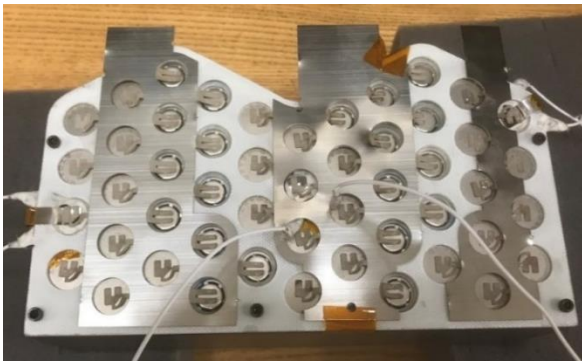
Figure 2. Photo of battery brick as prepared for testing.
