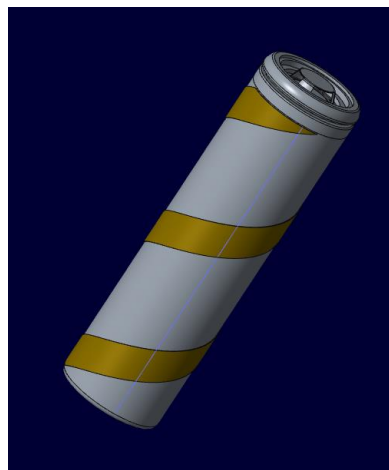
Figure 5. Spiraling mica paper wrapped around an 18650 cell.
