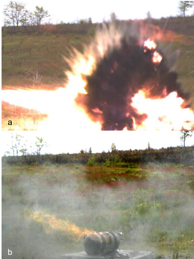
Figure 3: RPG impact: (a) the initial detonation of the RPG with initial jet, (b) flame tail sustained briefly after RPG penetration.
