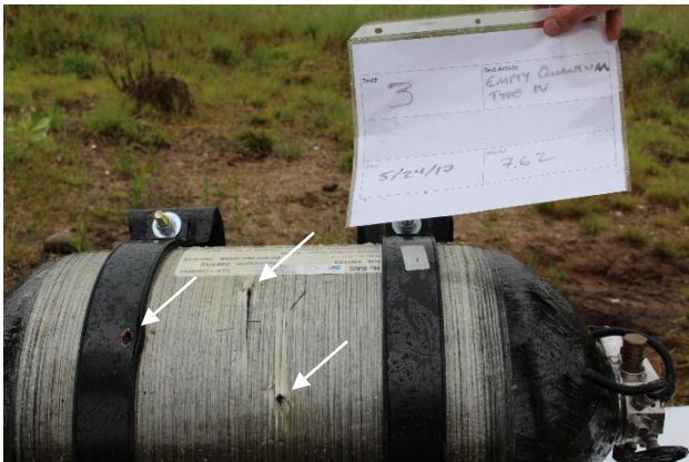
Figure 1: Control cylinder after three initial test shots. The arrows indicate where the rounds hit the cylinder.
