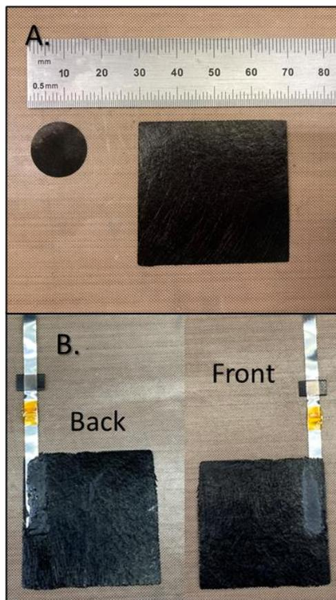
**Figure 1.** CNFP electrodes in different shapes. (A) The stiff carbon fiber framework allows the CNFP to be cut into different shapes and used for any number of cell geometries. (B) For use in the pouch cell, an aluminum tab can be glued directly to the CNFP without the need for a metal current collector.
