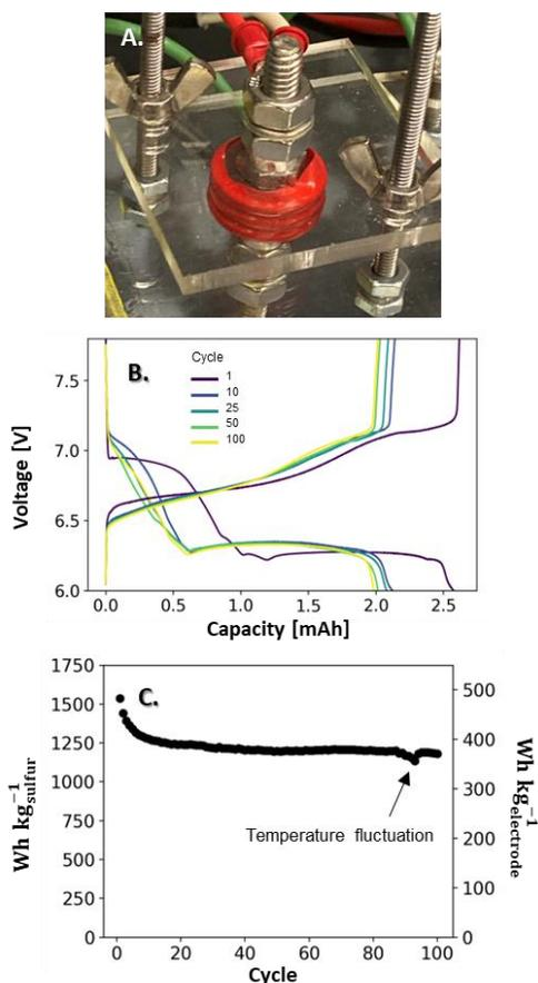
**Figure 2.** Three S@CNFP coin cells in series. (A) Coin cells can be placed in series to produce a high voltage Li-S system. Here, three coin cells are stacked to generate a system capable of >7.0 V. (B) Voltage profiles at various cycles and (C) cycling capacity are also shown.
