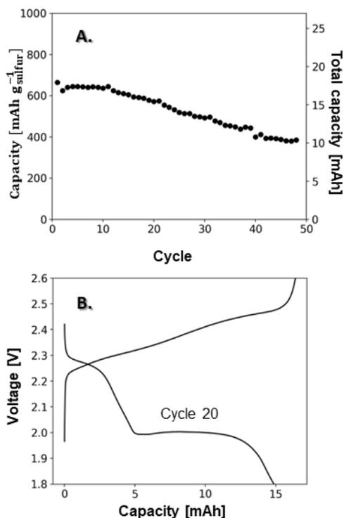
**Figure 3.** Electrochemical data for a pouch cell fabricated from a full sheet of S@CNFP. No metallic cathodic current collector was used in this cell. (A) Cycling data for ~50 cycles and (B) a representative voltage profile taken from cycle 20 detail the performance of the pouch cell.
