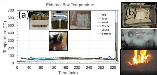
**Figure 4.** (a) External box temperature showing delayed thermal event within the box. Inset shows test article preparation and placement within secondary container and fire at the end of the test. (b) Pictures showing placement of test article within the secondary container and pressurized gas release and fire due to a lack of venting mechanism in the secondary box.
