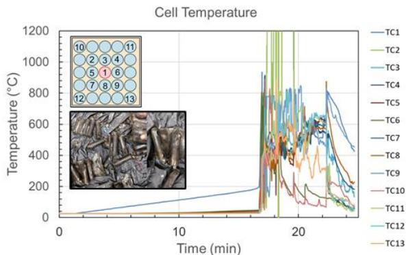
**Figure 2.** Cell temperatures and thermocouple layout for 100 % SOC test with interstitial material from manufacturer G. Inset shows post-test cell pictures with sidewall rupture.
