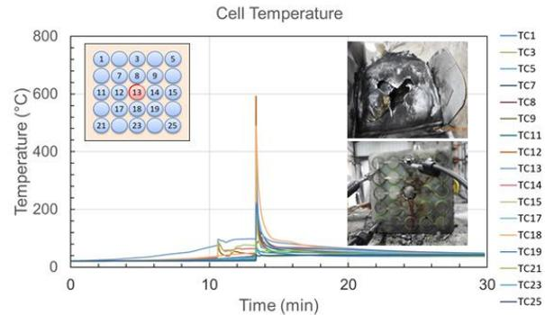
**Figure 3.** Cell temperatures and thermocouple layout for 100 % SOC 25P connected test with block material from manufacturer B.
