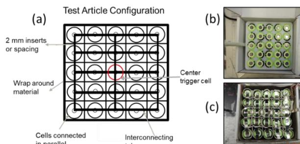
**Figure 1.** (a) Test article configuration showing the arrangements of 25 cells with trigger cell at the center of the configuration with inserts around each cell, (b) block-type phase change material and (c) combination of tubes and insert materials to separate 25P electrically connected cells in a shipping package.
